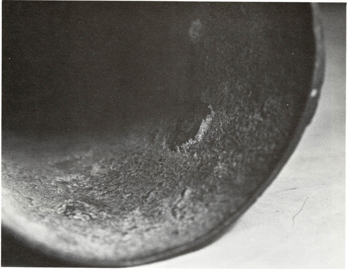
Pl. 6 — Keyed surface-chaplet, showing protrusion into bore.
