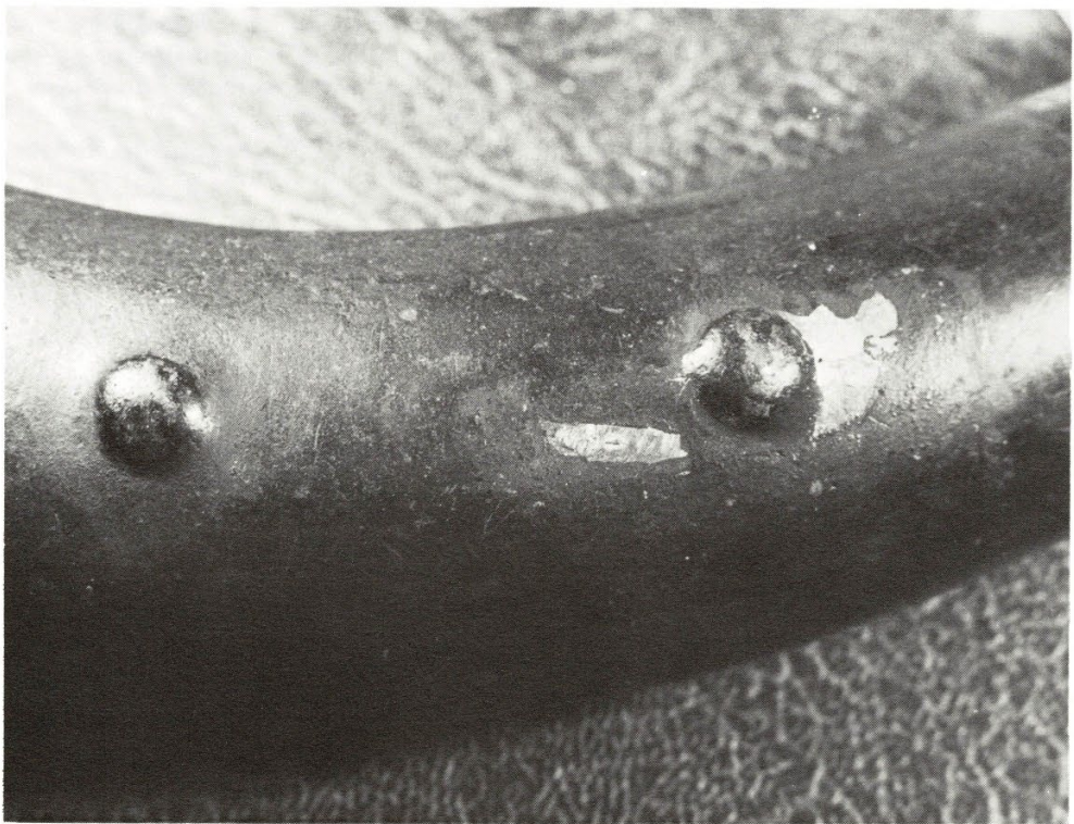
Pl. 2 — Cast-in features replacing apertures left by core-supports.
