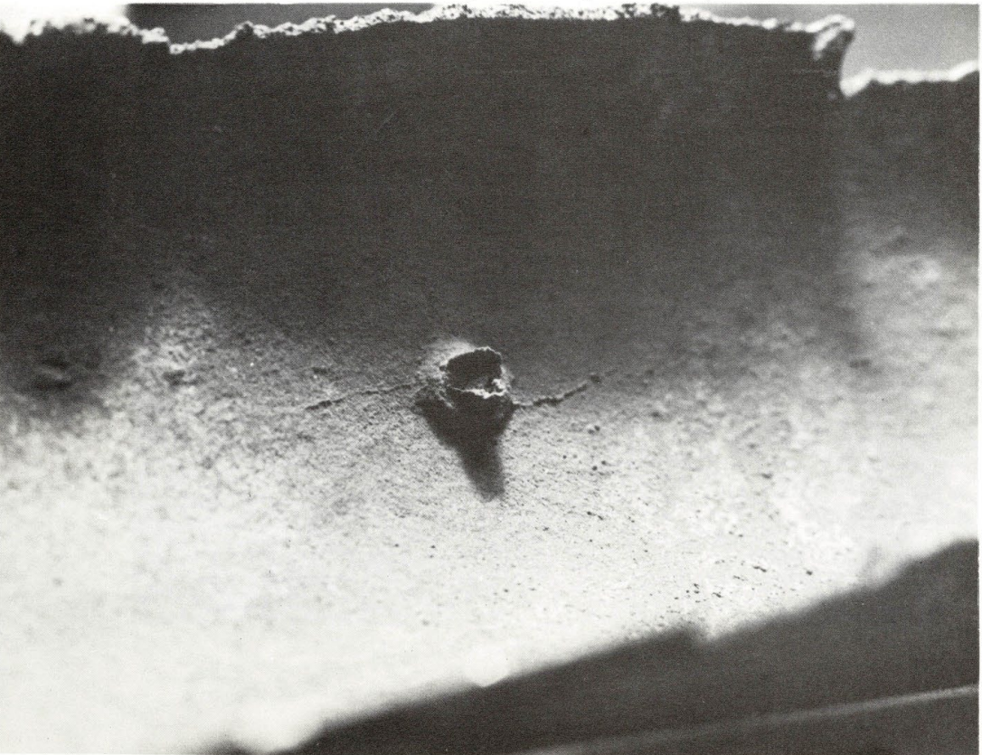
Pl. 9 — Tanged-chaplet protruding into bore.
