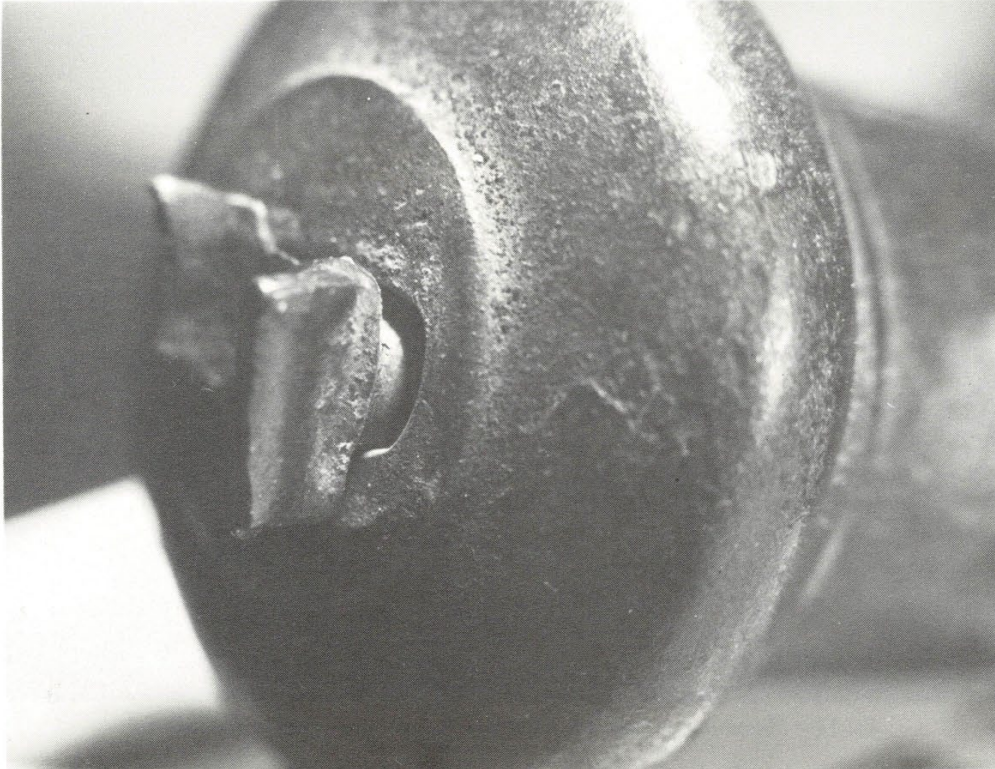
PL. 12 — Tip-mount showing wear from movement of mount.
