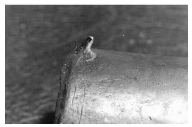
Plate 5.25a: A Cast-on Spike
