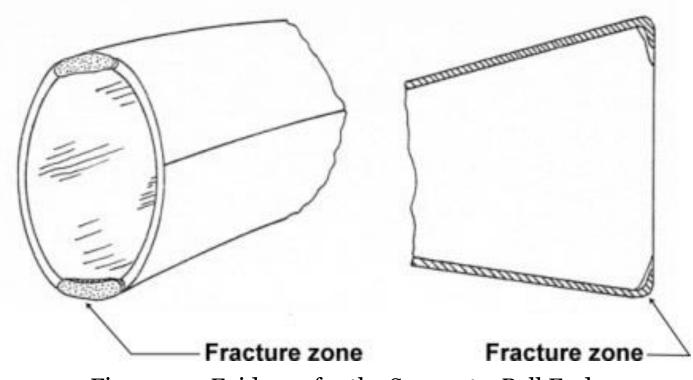
Figure 5.9: Evidence for the Sprue at a Bell End
