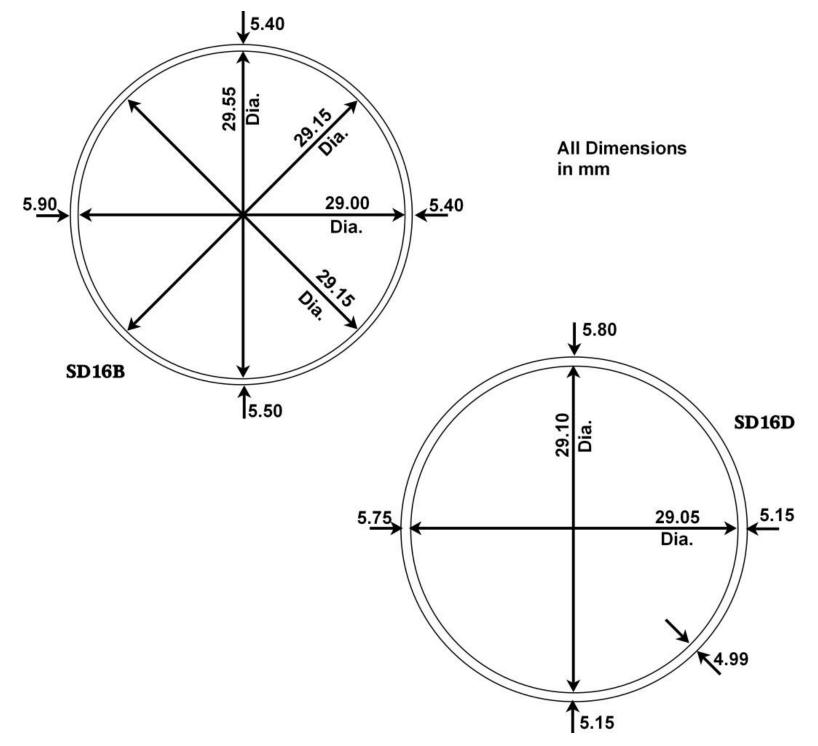
Figure 5.36: Dimensions of the Drumbest Carrying Rings
