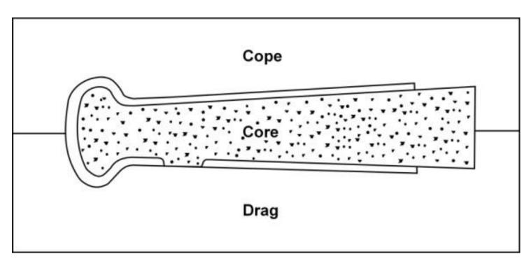
Fig 5.15: The Core-Support System for a Simple End-Blown Horn
