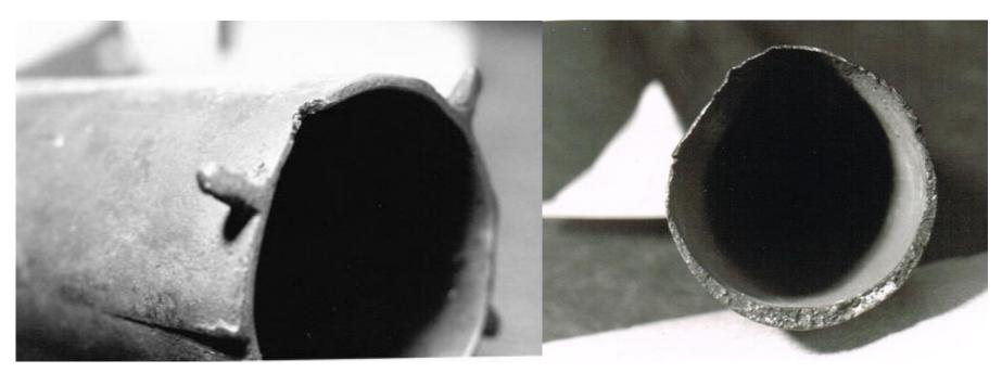
Plate 5.10: Registration Errors on Bell Ends And Broken-off Sprue Endings
