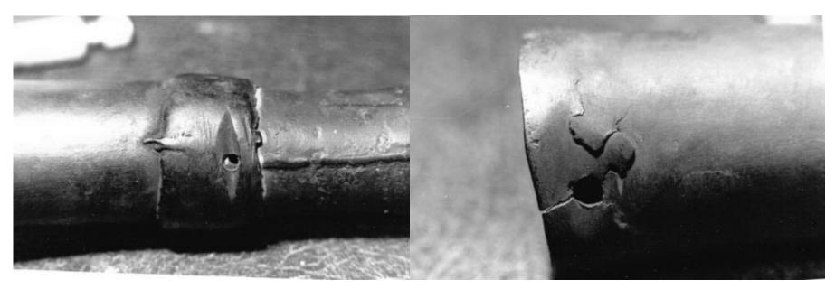
Plate 5.24: Post-Casting Work on Tubes
