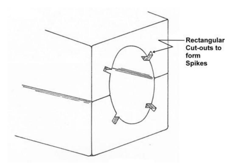
Figure 5.40: Forming the Spikes on a Bell End
