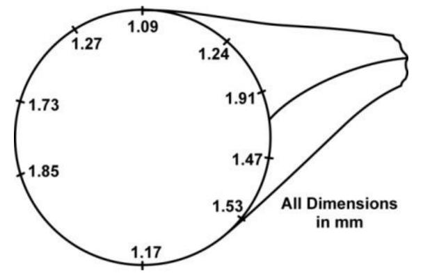
Figure 5.24: Measured Wall Thicknesses on Instrument SD32
