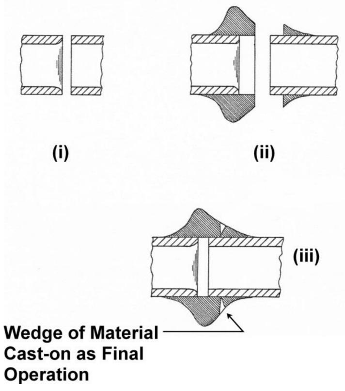
Figure 5.38: Joining together of the Drumbest End-Blow Instruments
