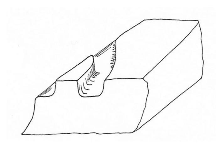
Figure 5.28: Creating an Integral Carrying Loop
