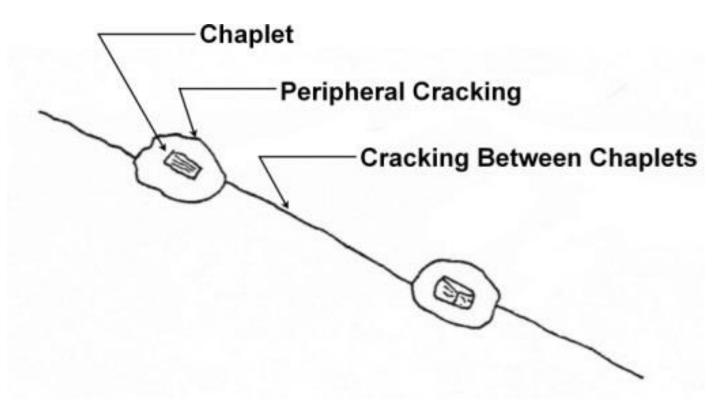
Figure 5.23: Cracking of the Core Around a Tanged Chaplet
