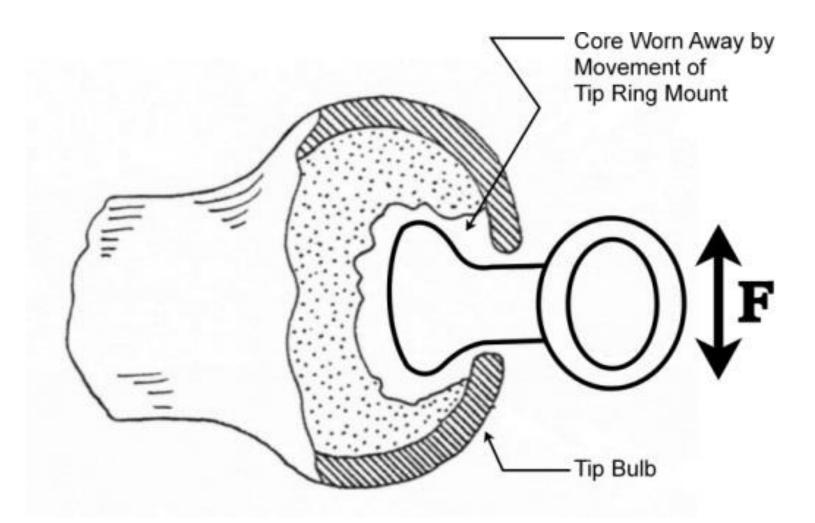
Figure 5.31: A Cast in Tip Ring Mount
