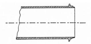
Figure: 5.5: A Bell-end Cross-Section
