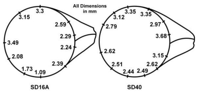
Figure 5.25: Measured Wall Thicknesses on SD16A and SD40
