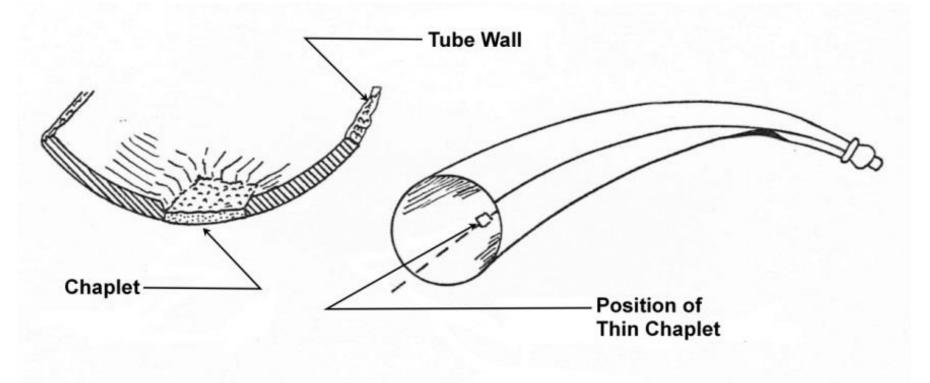
Figure 5.3 Surface Chaplets in a Tube Wall
