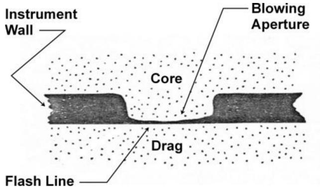
Figure 5.16: Possible Metal Flow Path over Blowing Aperture
