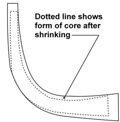
Figure 5.8(a): A Further Core Shrinkage Pattern
