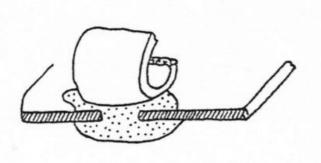
Figure 5.33: Attaching Tube Ring Mounts
