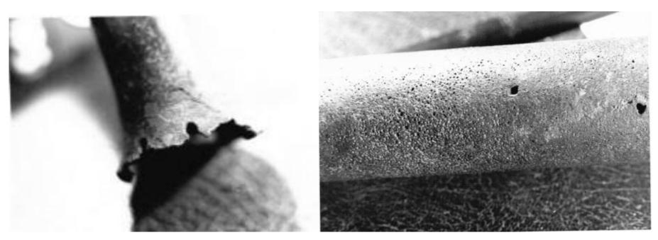
Plate 5.28: Post-Casting Work on a Tube and Tube Surface Finish
