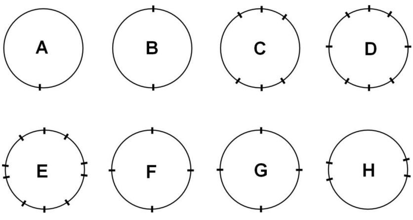
Figure 5.20: Different Chaplet Configurations
