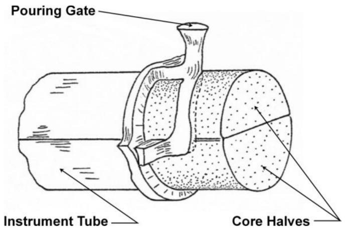
Figure 5.12:Gating Evidence on Bell Ends
