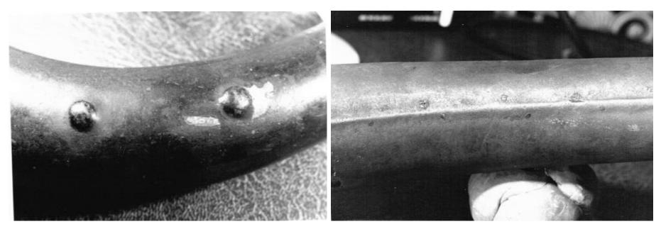
Plate 5.12: Chaplet Evidence on Tube Walls
