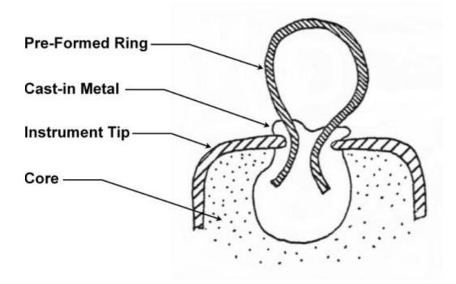
Figure 5.35: A Wrought Cast-in Ring Mount
