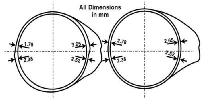
Figure 5.26: Measured Wall Thicknesses on SD19A
