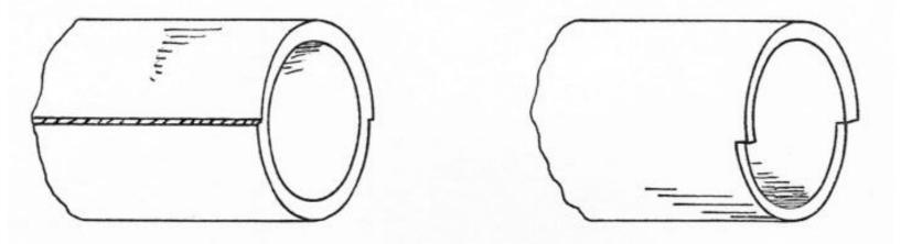
Figure 5.2a and 5.2b: Registration Errors in a Finished Casting
