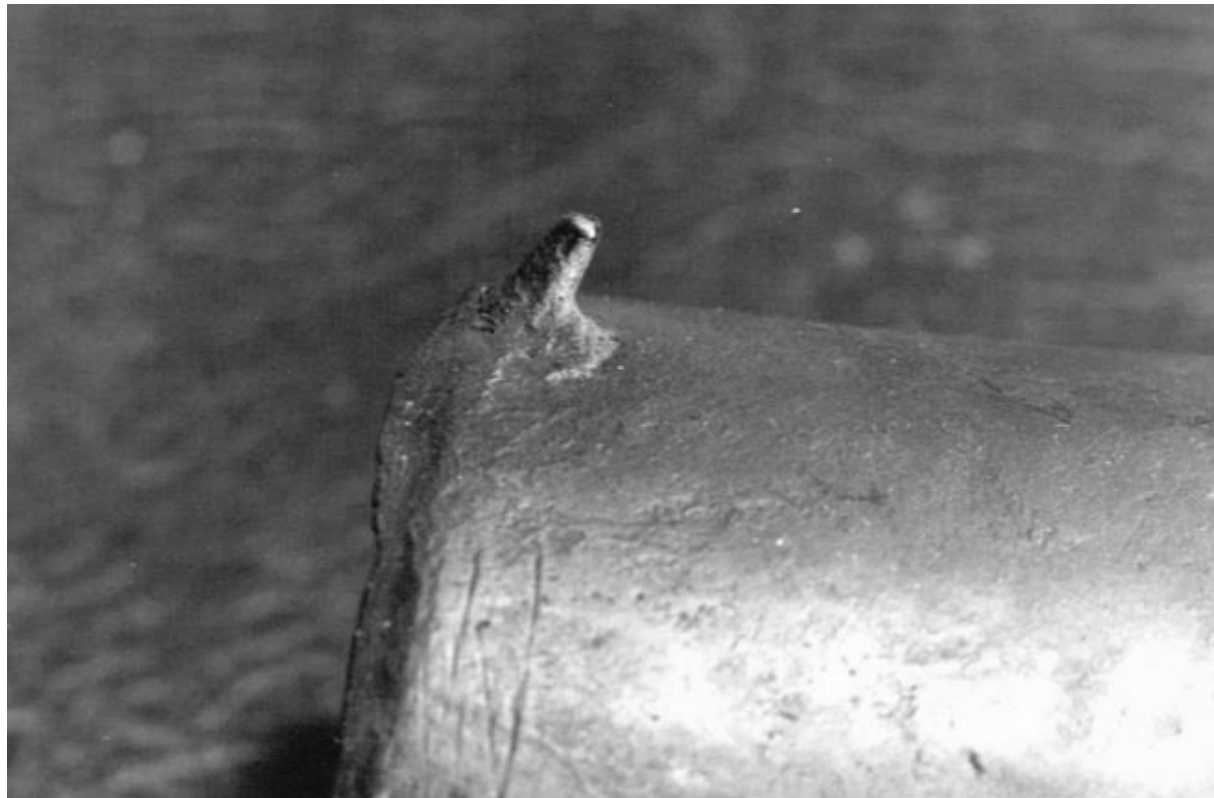
Plate 5.25a: A Cast-on Spike
