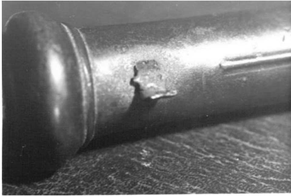
Plate 5.2(a): Chaplets, Carrying Rings and Casting Seams
