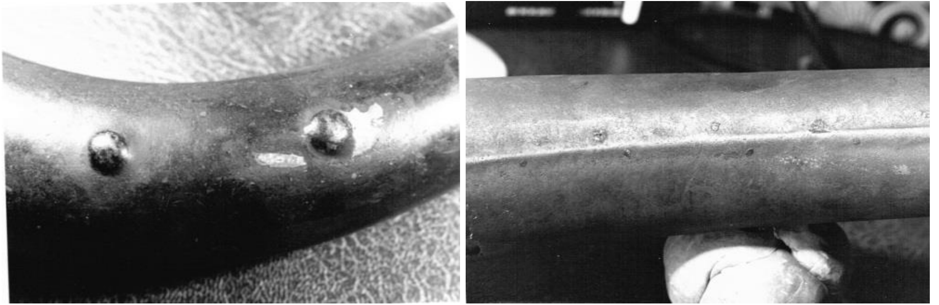
Plate 5.12: Chaplet Evidence on Tube Walls
